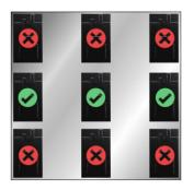
Polarization of Confidex Heatwave Tough is as shown below. This should be considered when using linear reader antennas.
