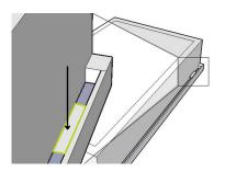
Ideal installation conditions are +20°C (+68°F) / 50% RH. For exceptional conditions, please contact Confidex. Adhesive of the label will provide best adhesion in 24 hours after the installation. Bond strength can be improved with firm application pressure.
